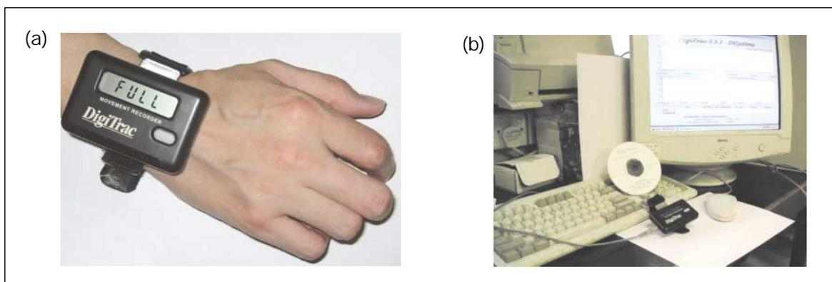
**Figure 1.** (a) The DigiTrac motion monitor is worn on the dominant hand before bed resting. It would continuously record wrist movements until the next morning. (b) The data is then downloading from the DigiTrac monitor to computer for analysis.
